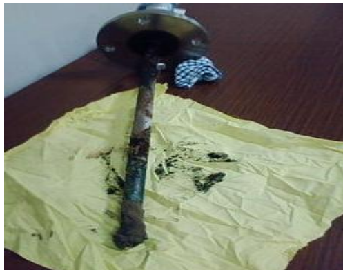
Fig.4 Non-coated thermo-couple damaged from tip of the same (図4 未被覆熱電対は先端部分が破裂した状態)
